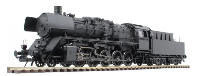
We requested last year to Lenz the manufacturing of a neutral black release of its BR 50, in order to have a simple base for a 1-150Z de la SNCF, a typical locomotive of the post WW2 era. The boiler is the former one and equipped with 1 steam dome and 2 sand domes.
