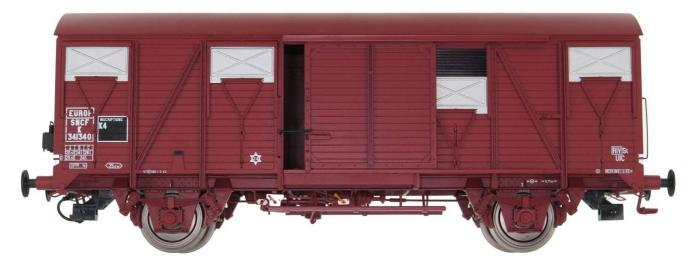
All wagons now take advantage of a clearly visible U-profiled underframe. Both doors and all flaps are functional and can be set in opened or closed states.
